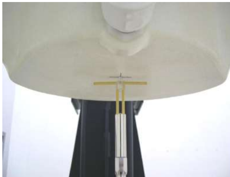
Picture 8.2 Photo of Dipole Setup
