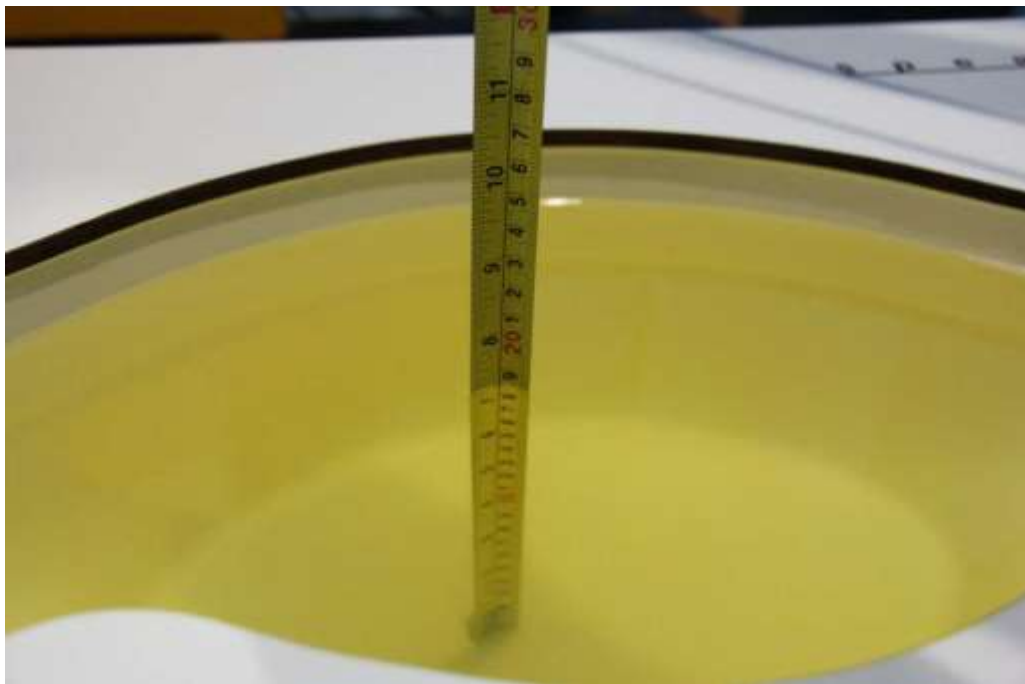
Picture 7-1: Liquid depth in the Flat Phantom(2450MHz)
