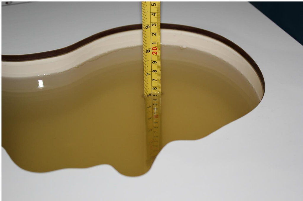
Picture 7-5: Liquid depth in the Head Phantom(2550MHz)
