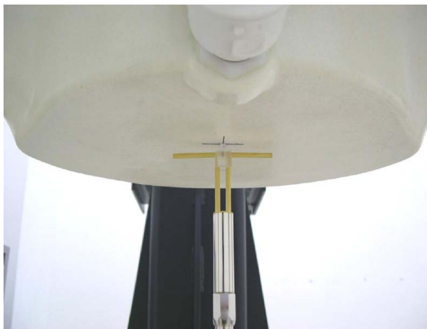
Picture 8.2 Photo of Dipole Setup
