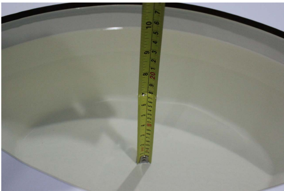
Picture 7-16 Liquid depth in the Flat Phantom (5GHz)
