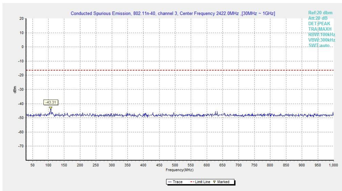
Fig.A.6.1.74 Transmitter Spurious Emission - Conducted (802.11n-HT40, Ch3, 30 MHz-1 GHz)
