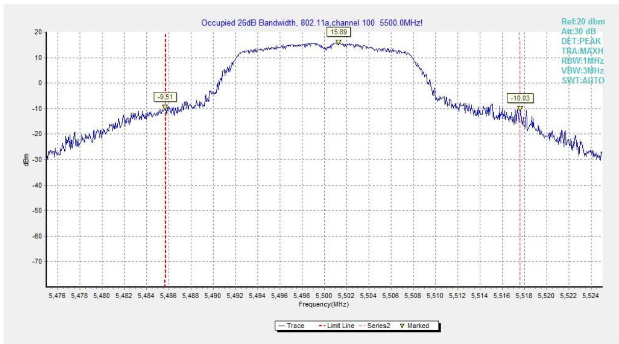
Fig. 7 Occupied 26dB Bandwidth (802.11a, 5500MHz)
