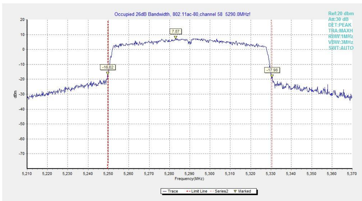
Fig. 42 Occupied 26dB Bandwidth (802.11ac-HT80, 5210MHz)
