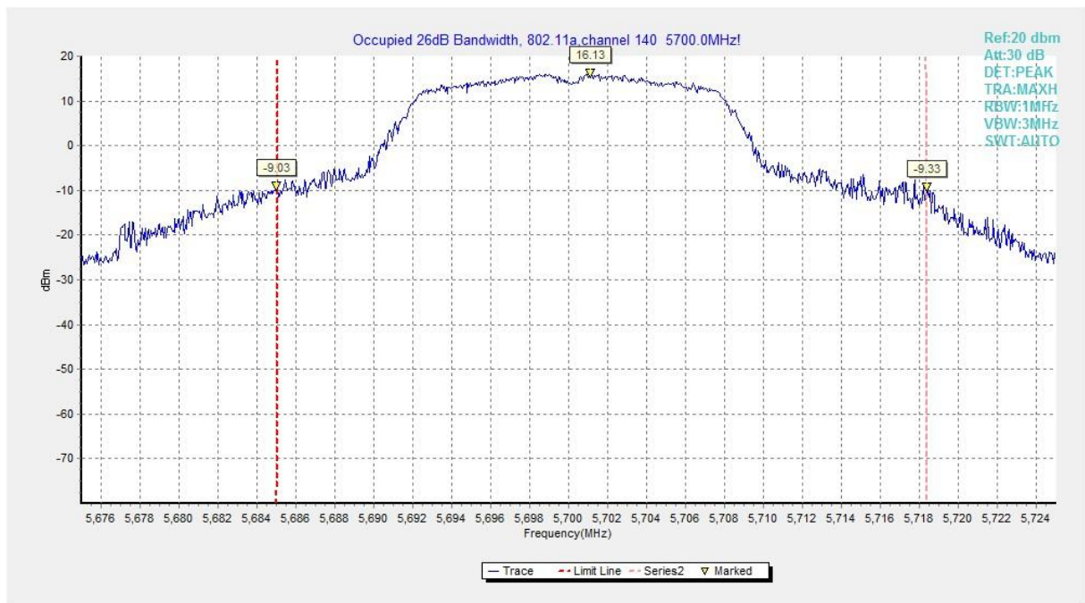
Fig. 9 Occupied 26dB Bandwidth (802.11a, 5700MHz)
