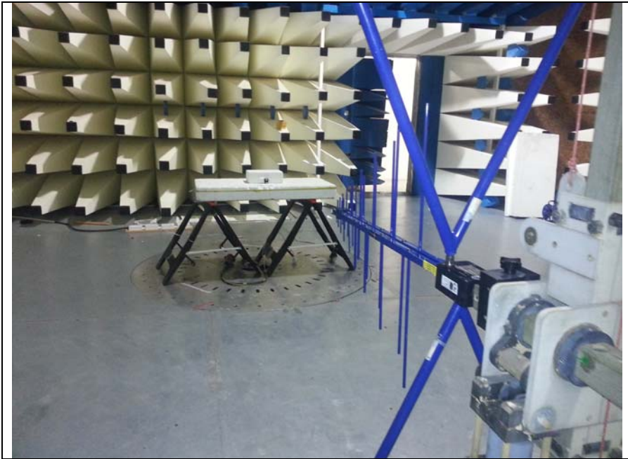
Fig 1 Test setup Rad Emissions
