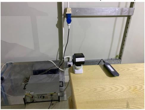
Radiated Emissions (30MHz-1GHz) Test Setup
