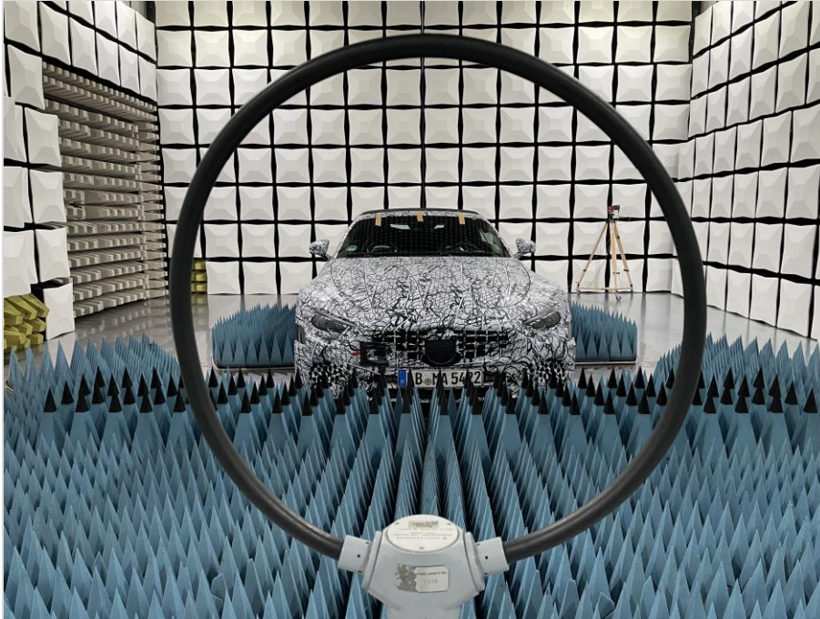
Photograph 1: EUT test setup, radiated field strength emissions below 30 MHz
