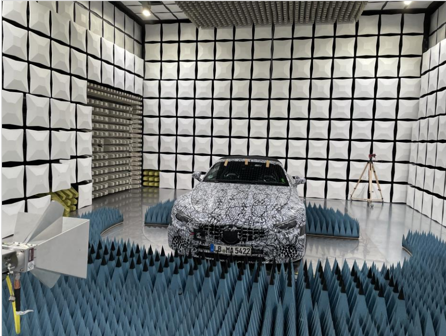
Photograph 3: EUT test setup, radiated field strength emissions above 1 GHz
