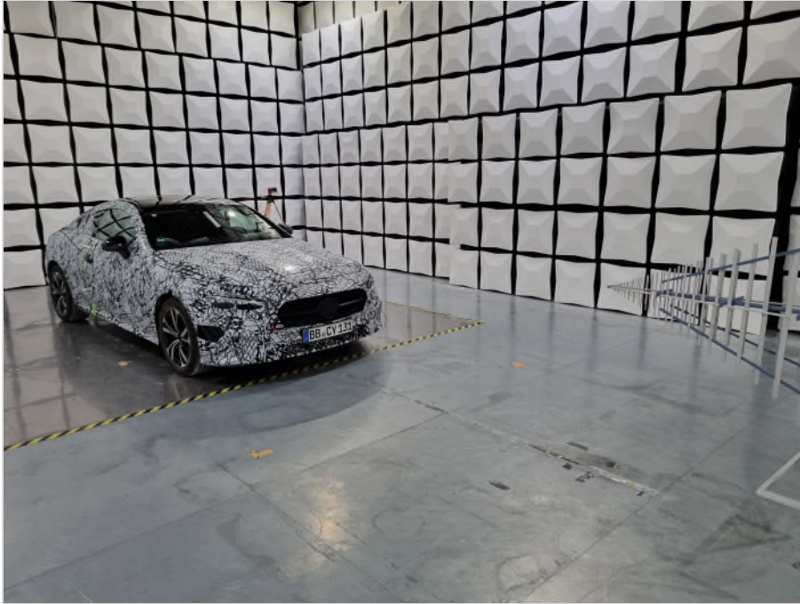
Photograph 1: EUT test setup for measurement < 1 GHz in the anechoic chamber, overview
