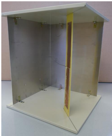
Replacement antenna (Dipole) for 434 MHz Antenna Gain -5 dBi
