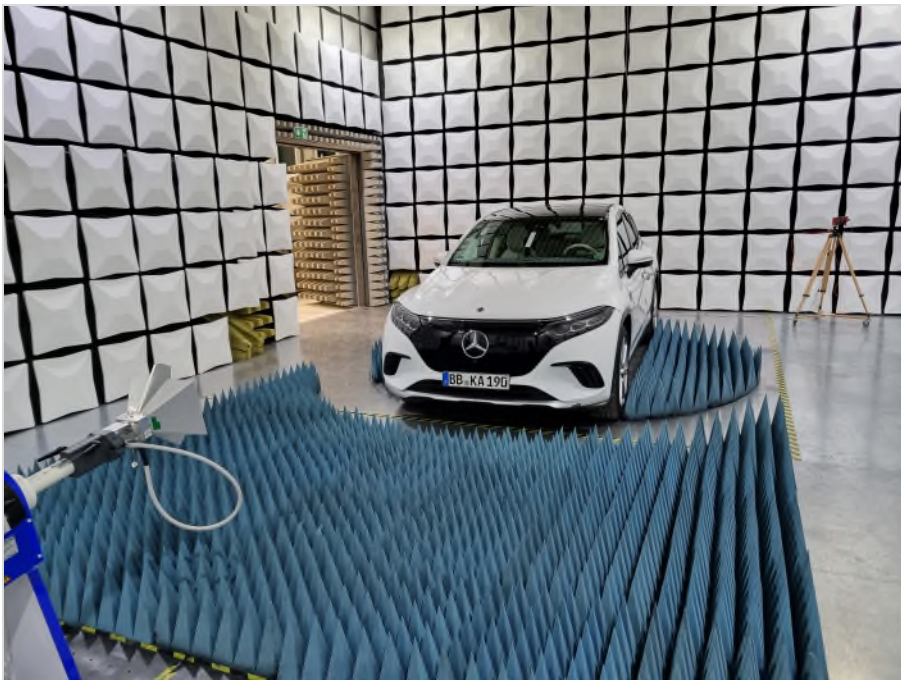
Photograph 2: EUT test setup for measurement > 1 GHz in the anechoic chamber, overview
