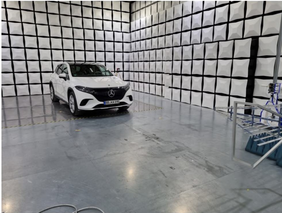
Fig. 5: Set up with EUT for test without absorbers at a car (EQS SUV (X296))
