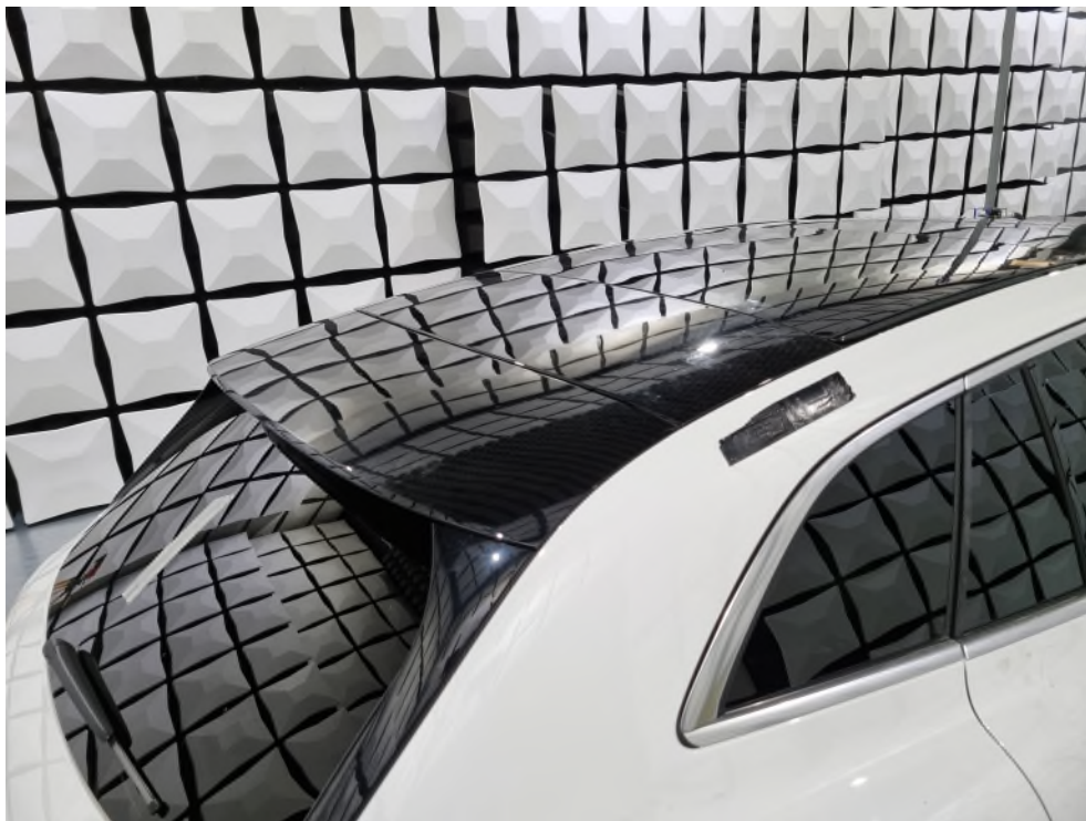
Fig. 6: EUT support details: set up when measuring the real antenna installed at the car (with cover)
