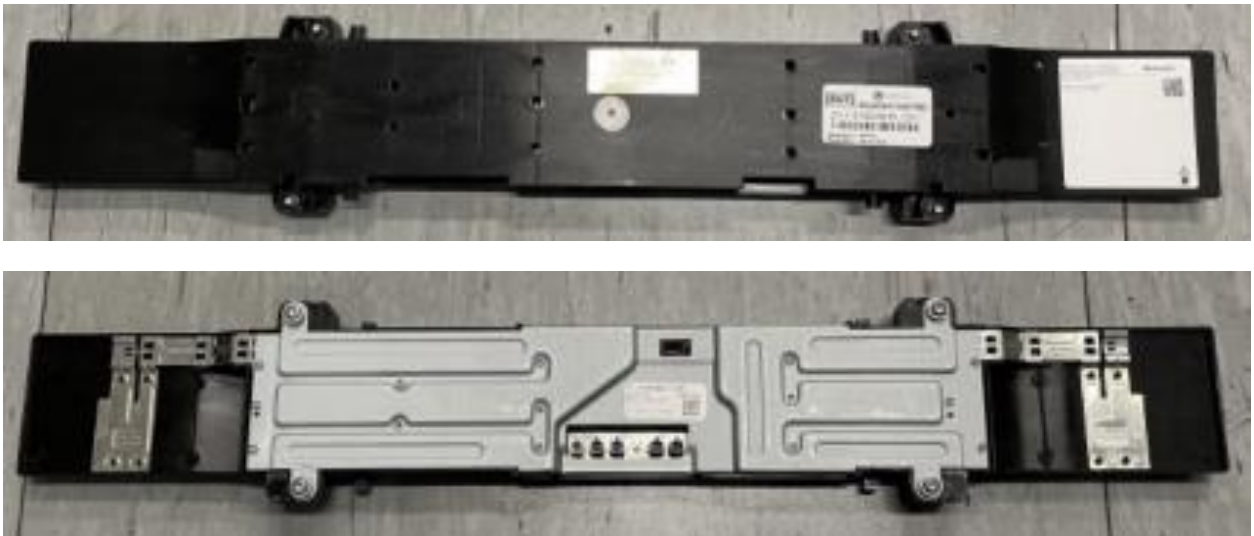
Top and bottom view of the real Telematics Module
