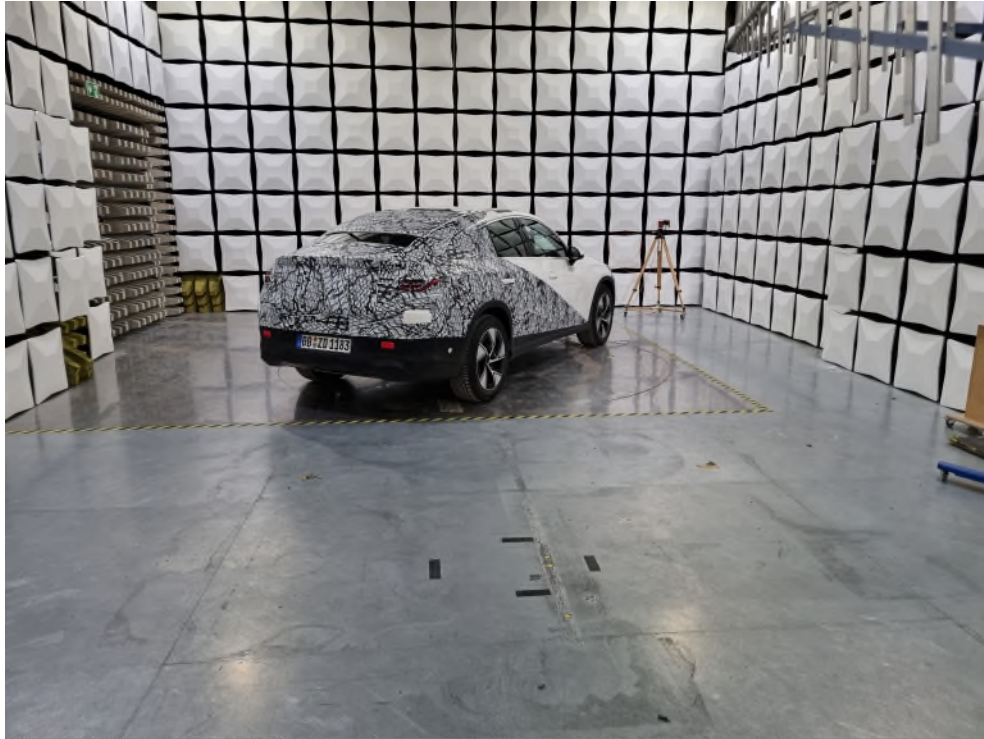
Fig. 5: Set up with EUT for test without absorbers at a car (C-Class (C254))
