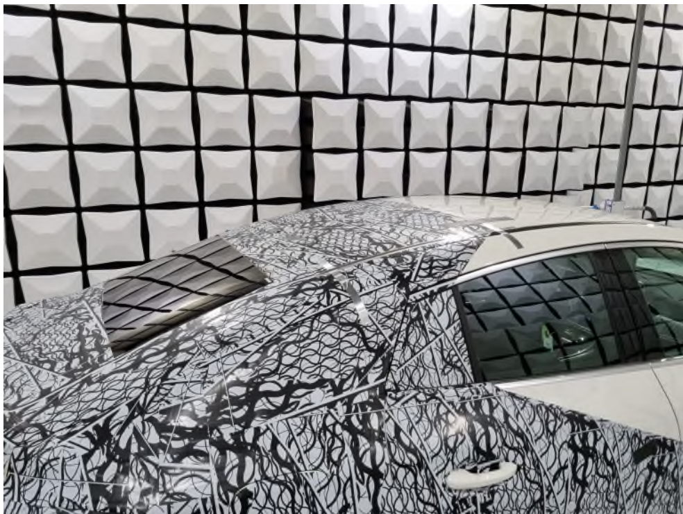
Fig. 6: EUT support details: set up when measuring the real antenna installed at the car
