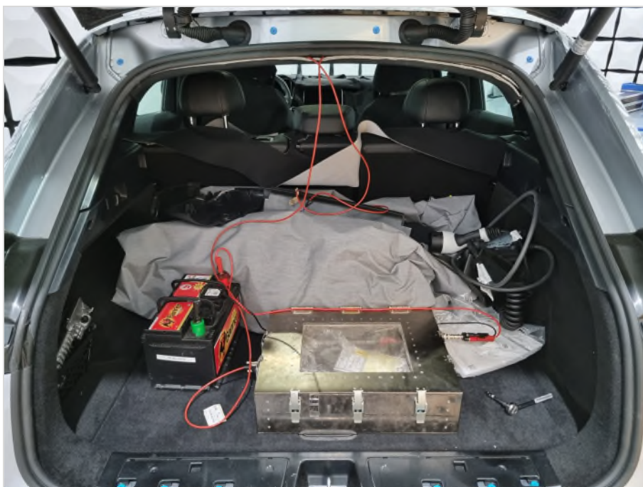
Photograph 4: Placement AE1 inside shielded enclosure
