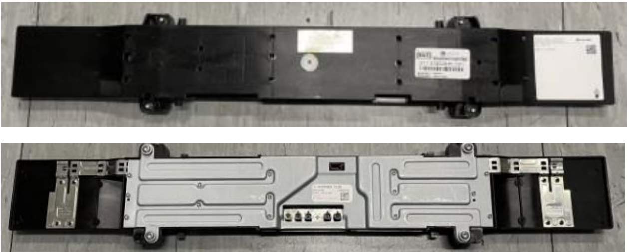
Top and bottom view of the real Telematics Module
