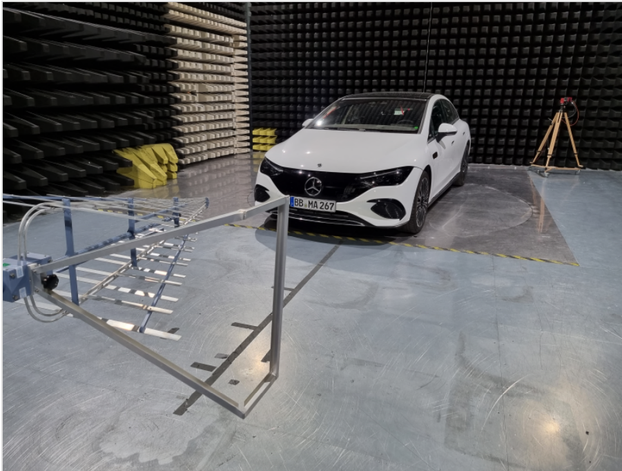
Photograph 1: EUT Test Setup in the anechoic chamber, Radiated field strength (< 1GHz)
