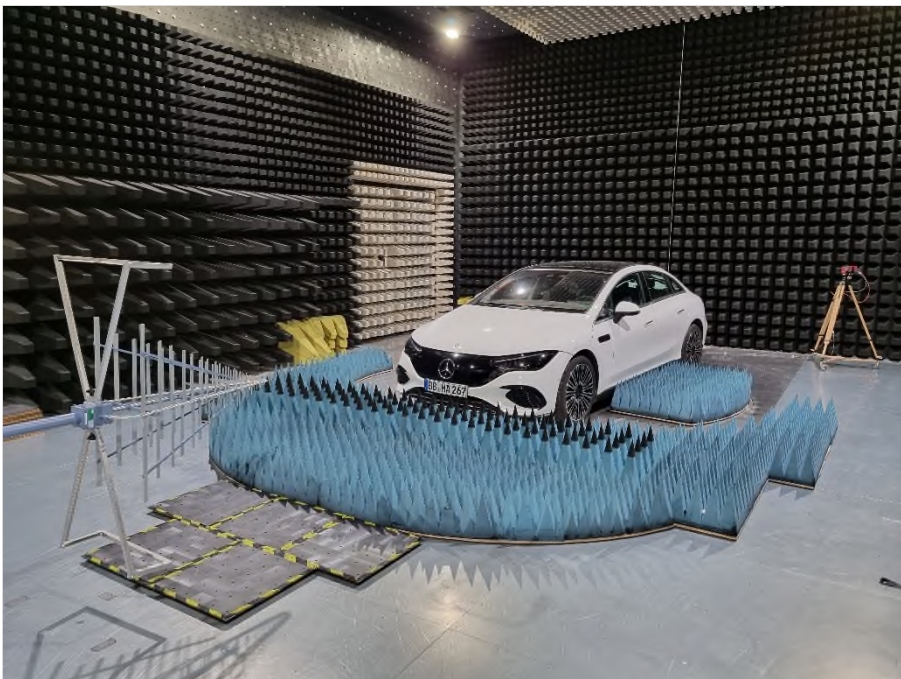
Photograph 2: EUT Test Setup in the anechoic chamber, Radiated field strength (> 1GHz)
