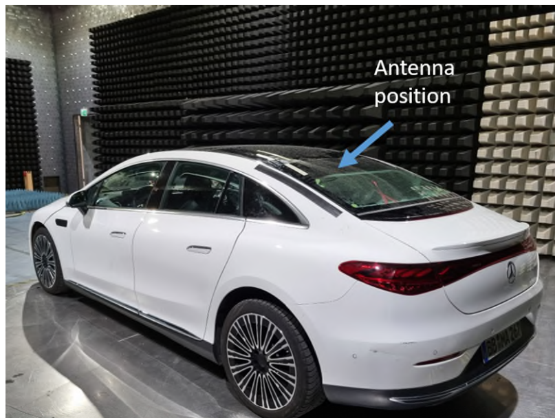
Fig. 3: Photo and indication of antenna position.
