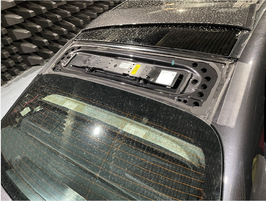
Photograph 3: AE 2 (Antenna placement)
