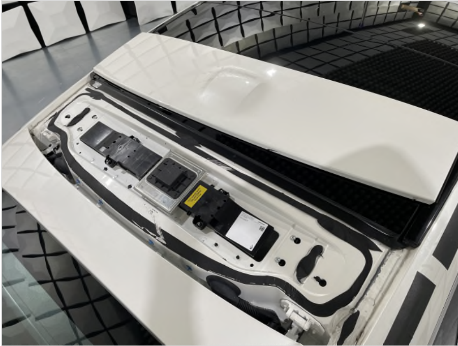
Photograph 3: AE 2 (Antenna placement)
