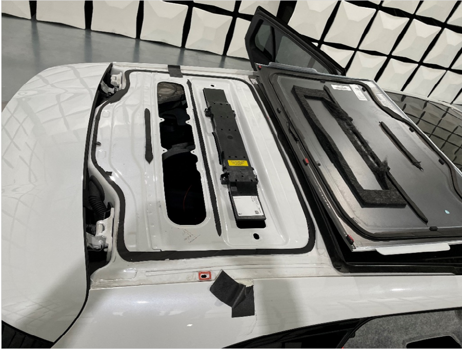
Photograph 3: AE 2 (Antenna placement)
