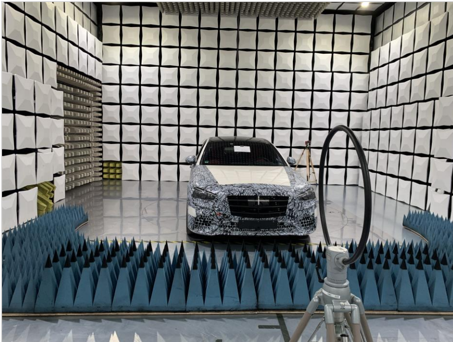
Photograph 3: EUT Setup Magnetic Field Measurements in the Semi anechoic chamber (9kHz to 30MHz frequency range)
