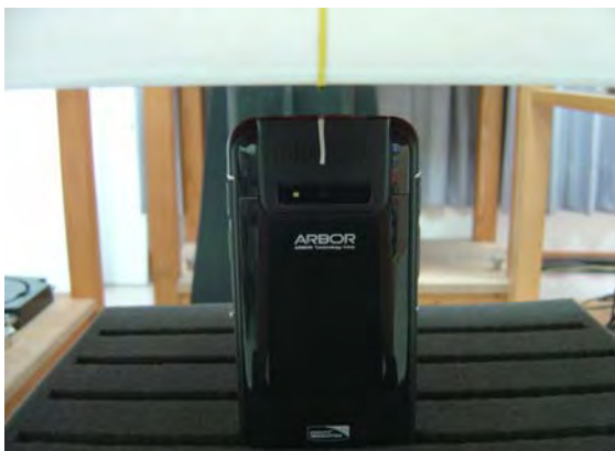
Fig.9 EUT top to flat phantom
