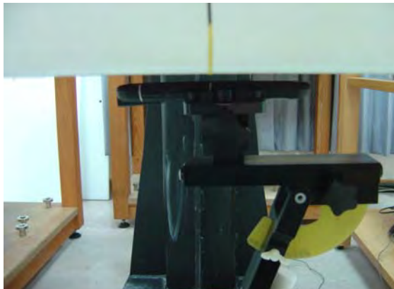
Fig.7 EUT front to flat phantom
