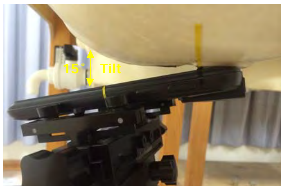
Fig.6 Left Head Section / Ear-Tilt Position(15°)
