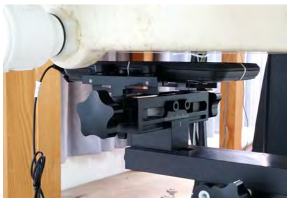
Fig.13 EUT front with headset to flat phantom
