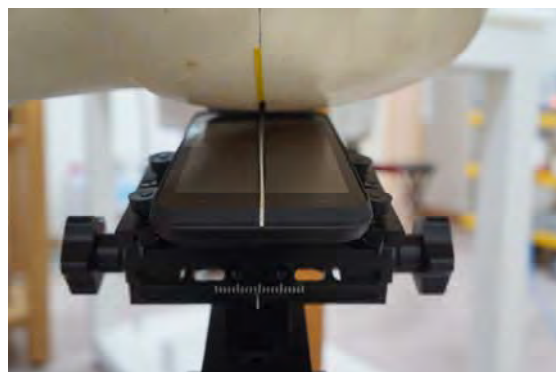
Fig.6 Left Head Section / Ear-Tilt Position(15°)
