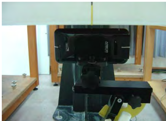
Fig.11 EUT right to flat phantom
