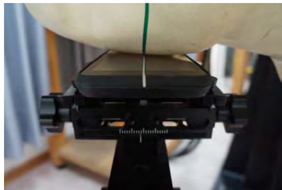
Fig.3 Right Head Section / Cheek-Touch Position
