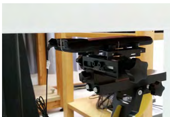
Fig.14 EUT back with headset to flat phantom
