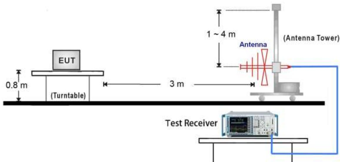
1GHz ~ 18GHz Test Setup:
