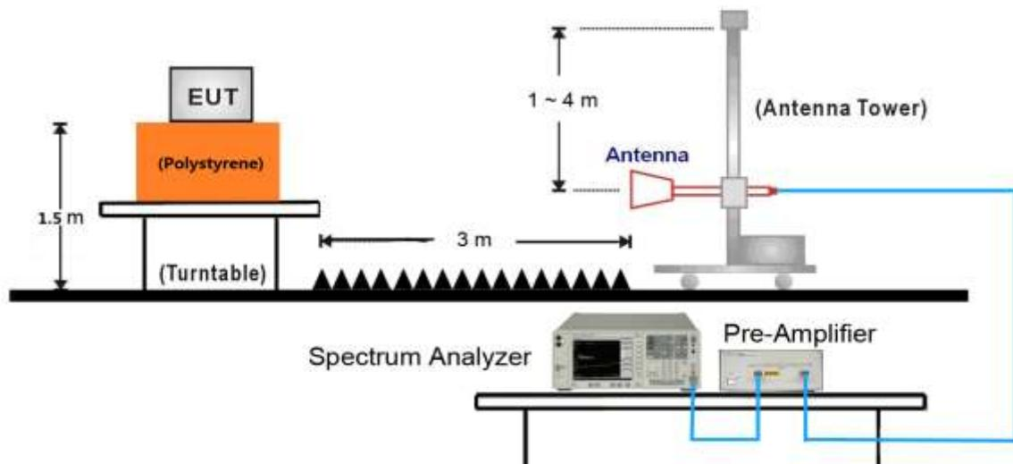
18GHz ~25GHz Test Setup:
