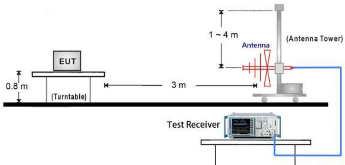
1GHz ~ 18GHz Test Setup:
