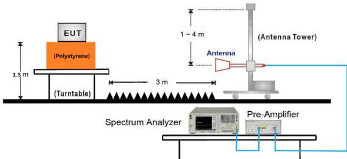
18GHz ~25GHz Test Setup:
