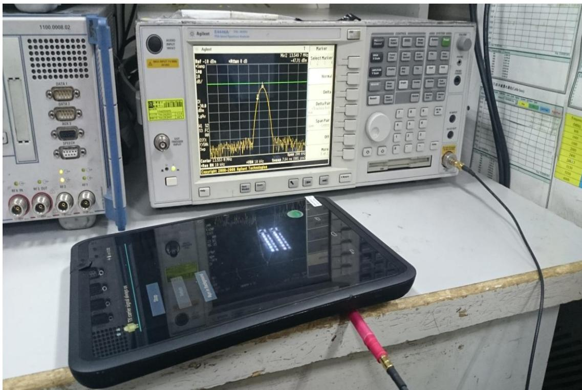
**Radiated Emission Set up Photos****9kHz ~ 30MHz**
