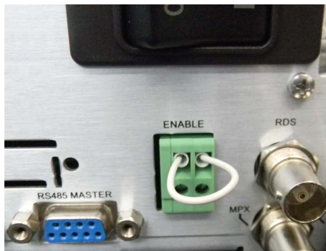
Fig. 8 – ENABLE short circuit (INTERLOCK)
