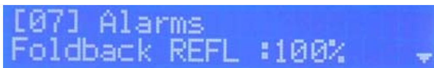
Fig. 20 – Set Fold back REFL
