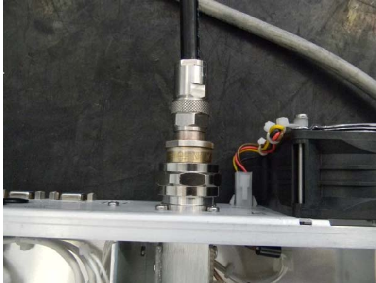
Fig. 7 – 50ohm load connection
