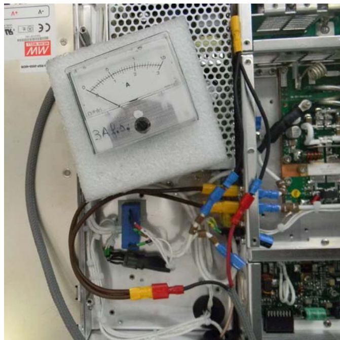
Fig. 10 – Amper-meter in series
