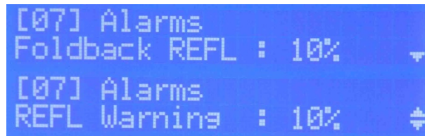
Fig. 25 – FOLD BACK REFL and REFL WARNING are set to 10%
