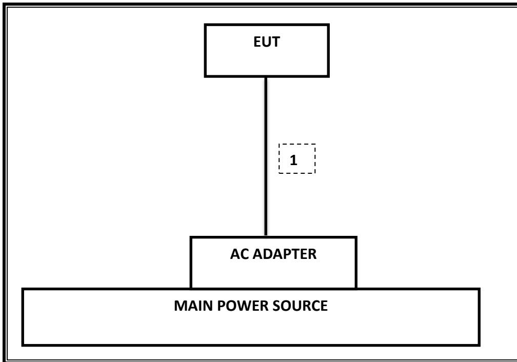
**SETUP DIAGRAM FOR AC LINE TESTS**
