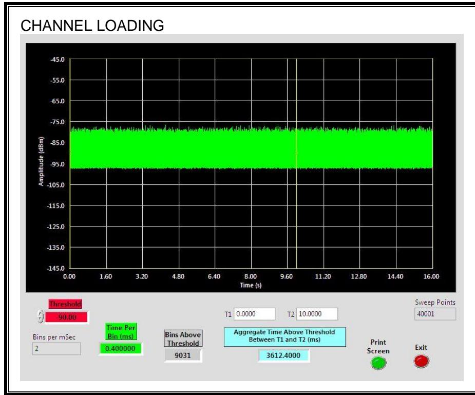
The level of traffic loading on the channel by the EUT is 36.12%
