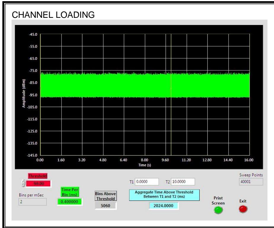
The level of traffic loading on the channel by the EUT is 20.24%
