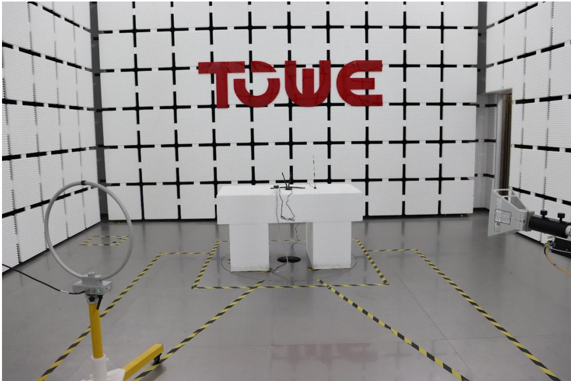
Field Strength of Spurious Radiation – 9kHz to 30MHz
