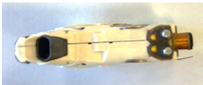
Picture 5 Radio module from bottom side
