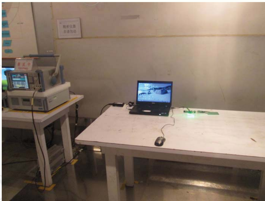
TEST SETUP OF CONDUCTED EMISSION
