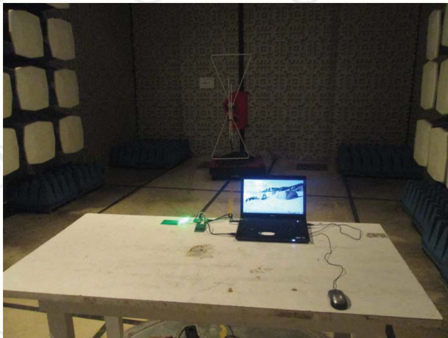
TEST SETUP OF RADIATED EMISSION (30MHz~1GHz)
