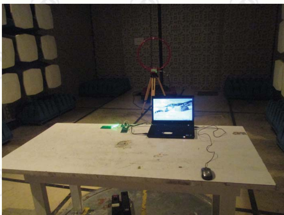
TEST SETUP OF RADIATED EMISSION (Below 30MHz)
