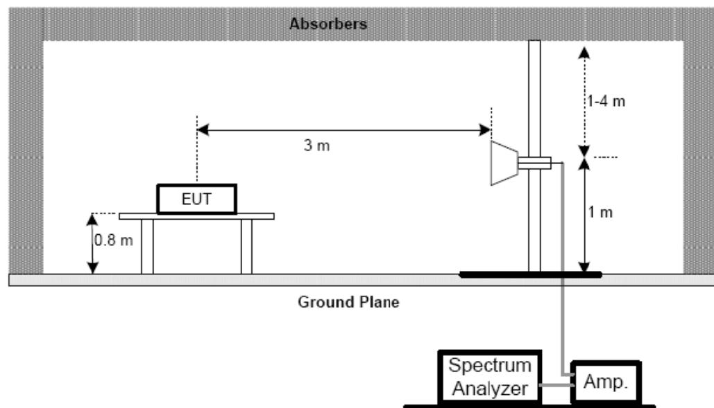
(C) For radiated emissions below 30MHz
