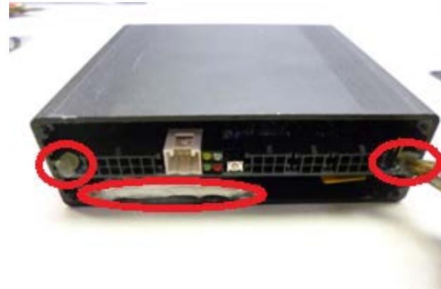
Use black screws (4pcs) to secure plate to chassis. Install wifi Antenna.
