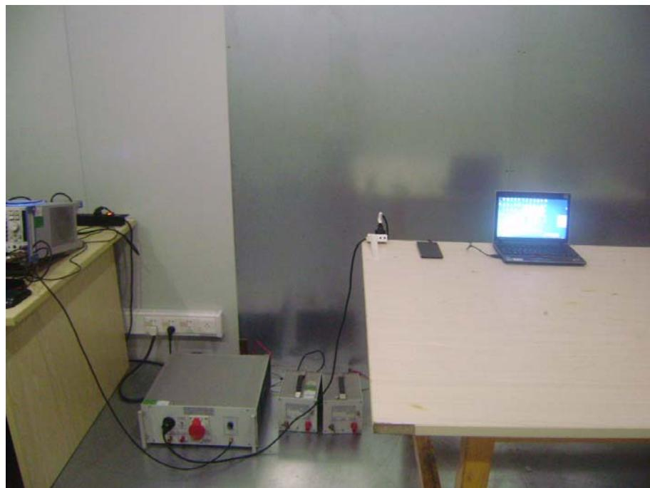
**Radiation Emission Test Setup (9 kHz to 30MHz)***Charging and Playing*
