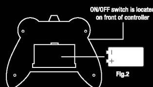
Radio controller uses one "9V" battery (not included).
