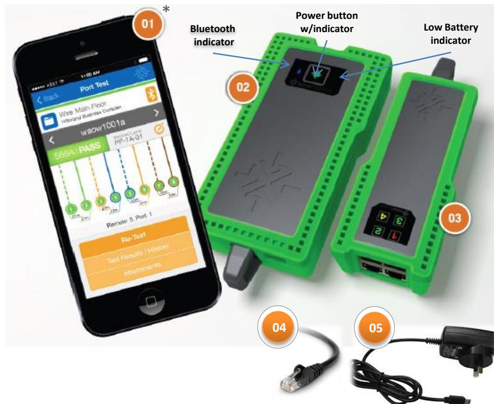
**01: WOWTester App:** This is a mobile application that acts as the “brains” of the testing components. The App works in conjunction with the other two components to run cable tests. The App initiates the tests and processes the test result data. \*
