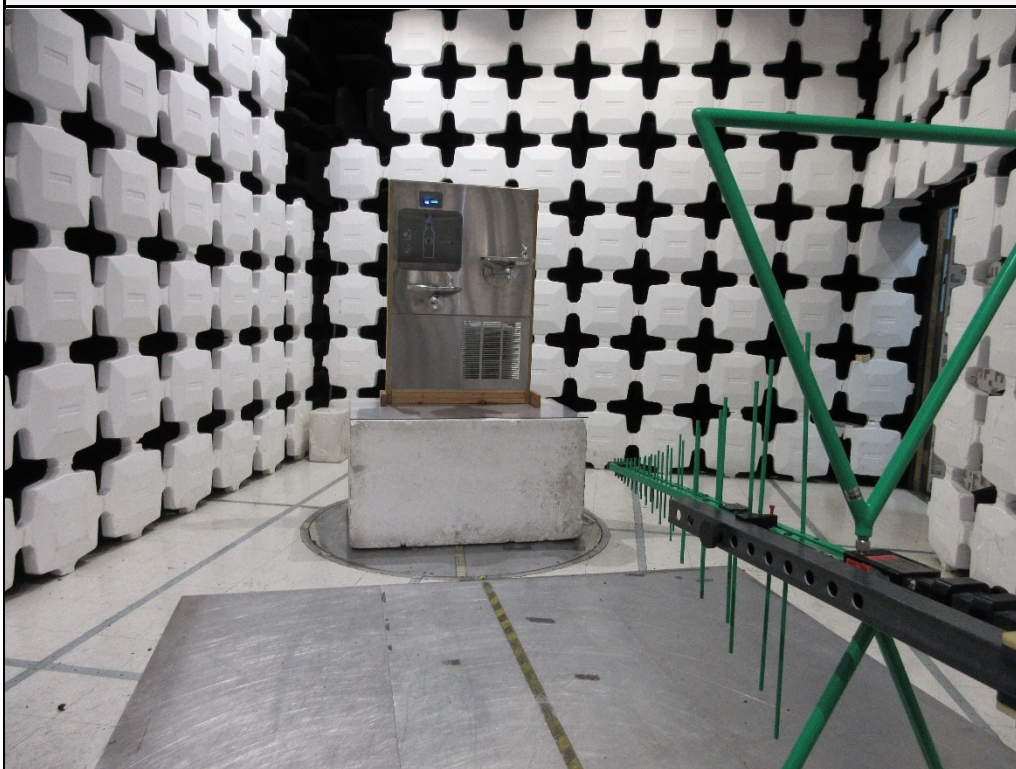
Test Setup for Spurious Radiated Emissions, Above 30-1000MHz – Antenna Polarization Vertical
