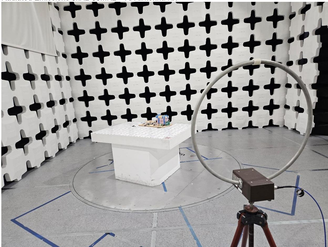
Radiated Emissions 9kHz-30MHz – RX antenna Hy
