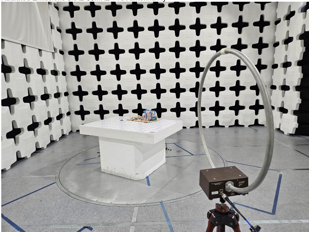
Radiated Emissions 9kHz-30MHz – RX antenna Hz
