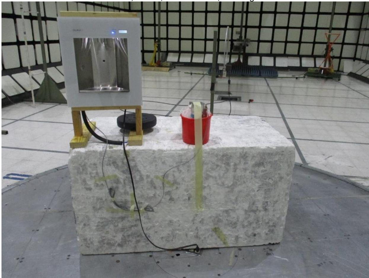
Radiated Emissions 30MHz-1GHz, Filter Inside
