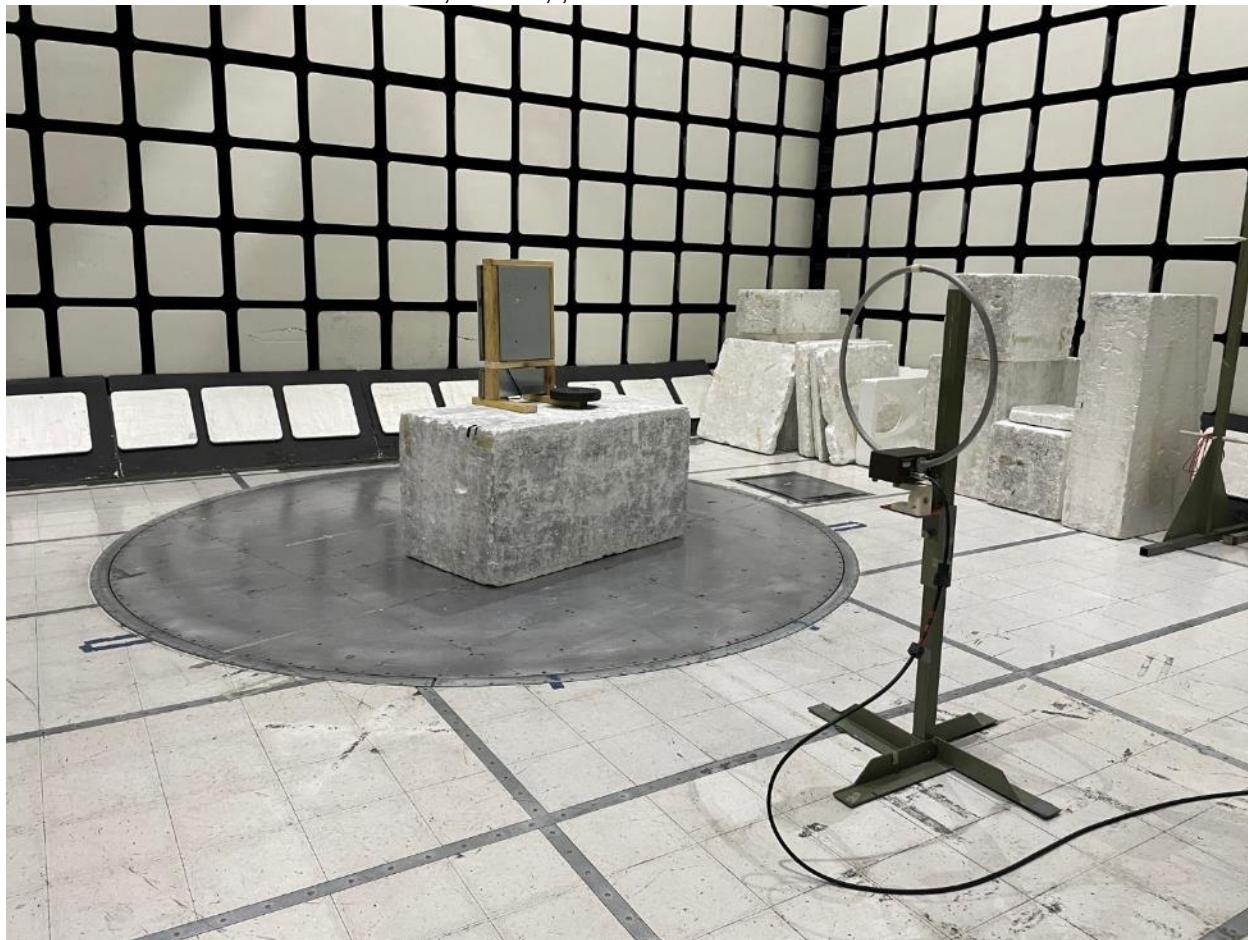
Radiated Emissions 9kHz-30MHz, Z-Axis, , Filter Inside
