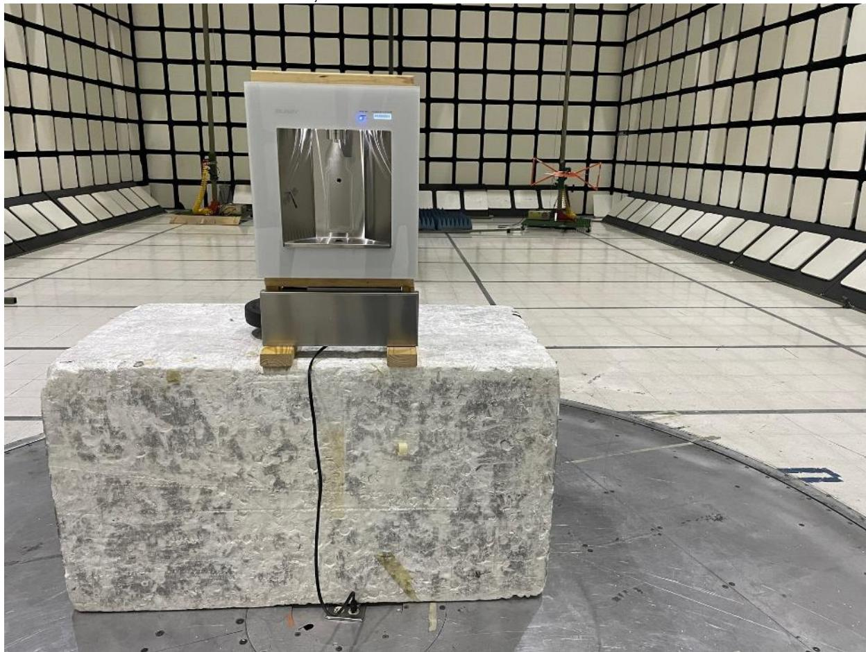
Radiated Emissions 30MHz-1GHz, Filter Remote
