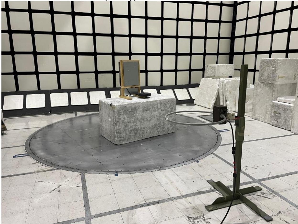
Radiated Emissions 9kHz-30MHz, Y Axis, Filter Remote, With tag
