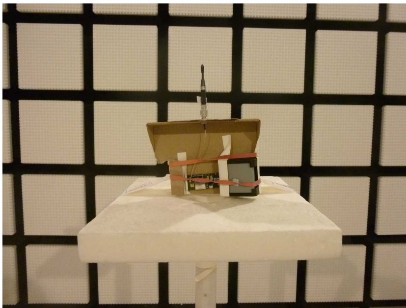
Photo 2: BTLE test setup in the anechoic chamber
