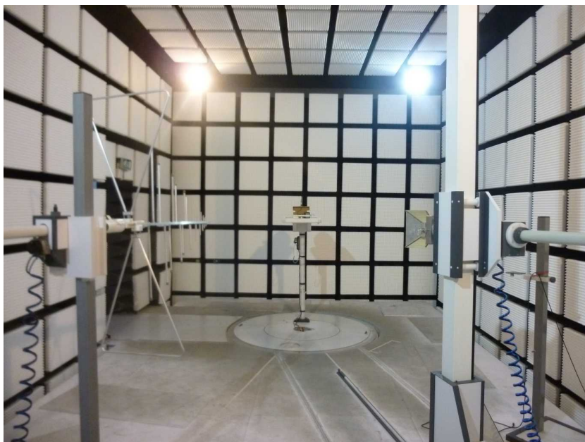
Photo 12: 902-928 MHz proprietary test setup at the anechoic chamber
