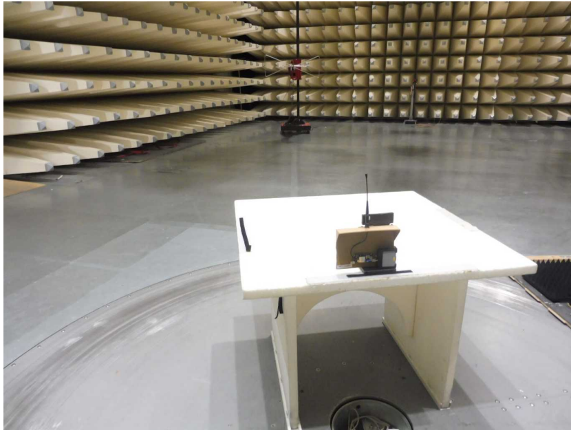
Photo 13: 902-928 MHz proprietary test setup at the semi-anechoic chamber
