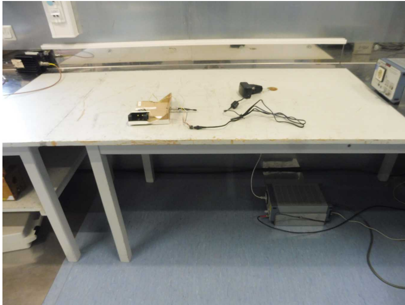
Photo 15: AC conducted emission test setup
