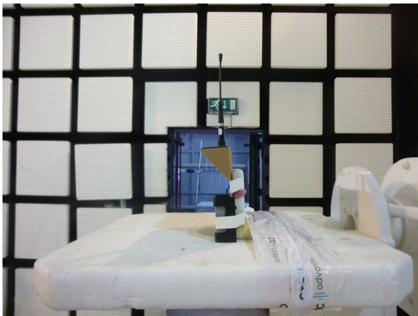
Photo 8: 902-928 MHz proprietary test setup at the anechoic chamber
