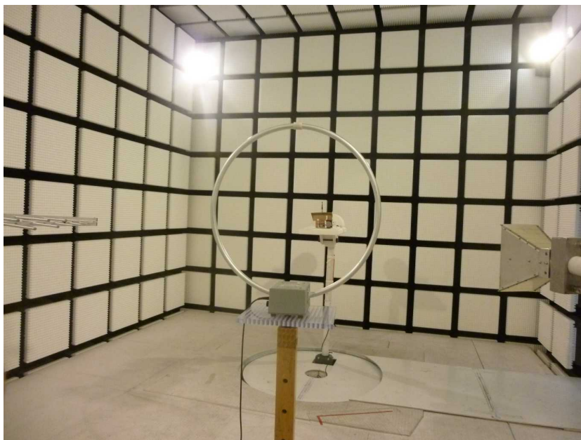
Photo 6: BTLE test setup in the anechoic chamber
