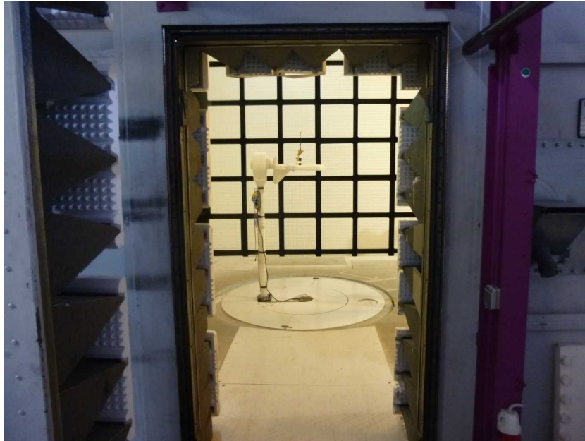
Photo 7: 902-928 MHz proprietary test setup at the anechoic chamber
