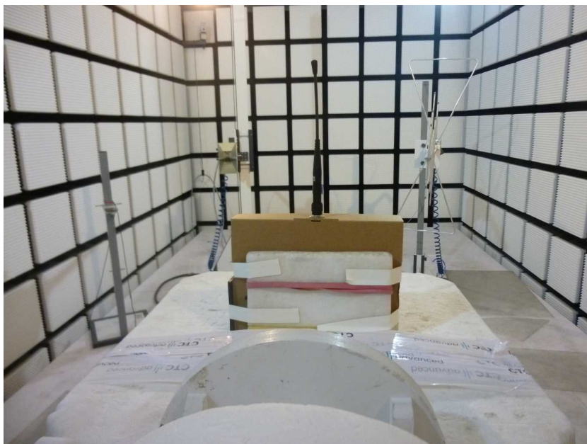
Photo 10: 902-928 MHz proprietary test setup at the anechoic chamber
