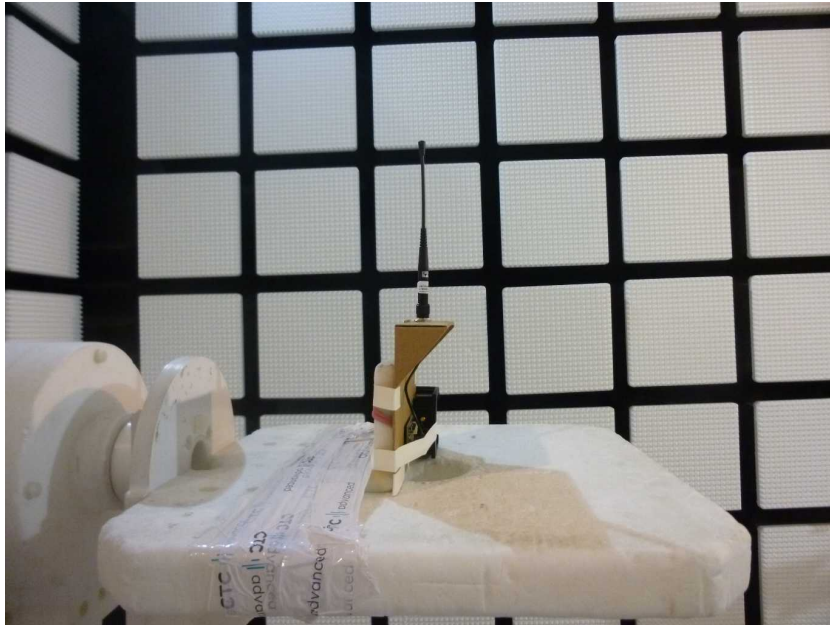
Photo 11: 902-928 MHz proprietary test setup at the anechoic chamber
