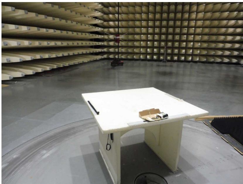
Photo 14: BTLE test setup in the semi-anechoic chamber
