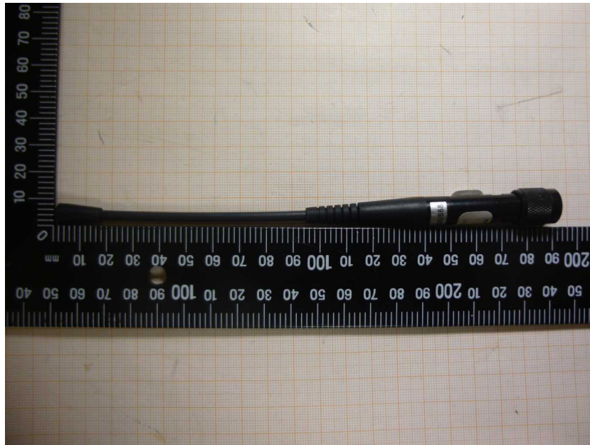
Photo 7: 902-928 MHz proprietary antenna
