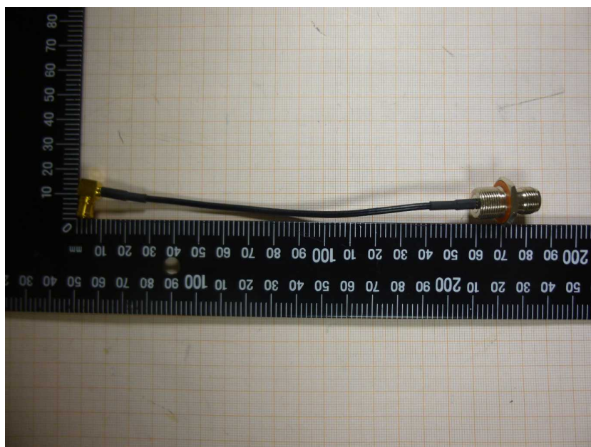
Photo 8: 902-928 MHz proprietary cable
