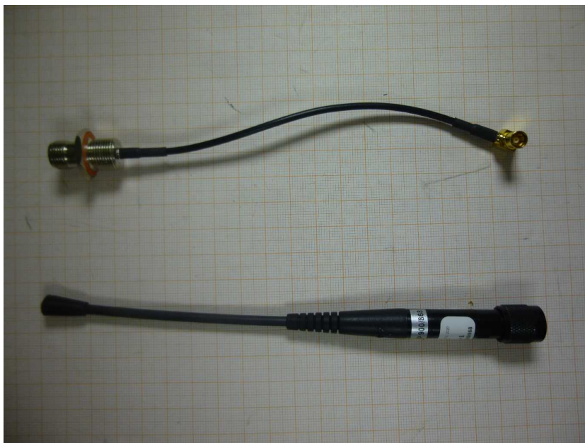
Photo 6: 902-928 MHz proprietary antenna and cable
