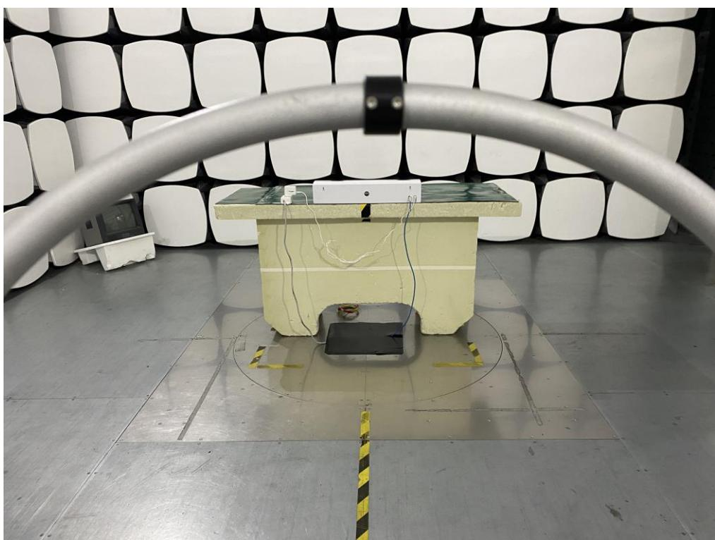
**Radiated Emissions Test Photos****30 MHz to 1000 MHz**
