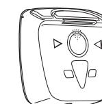
\* The batteries in your Smart-Reader can be replaced by simply removing the T-10 screw and lifting the front of the Smart-Reader off.
