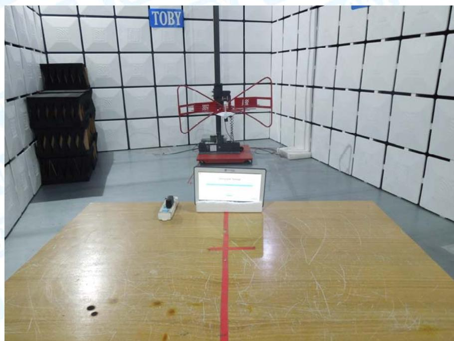
**Photo of Setup for Conducted Emission**
