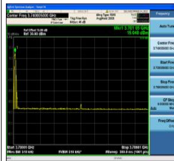
1-N77-3700-3980-PC2-30-80-L-4-CP-QPSK- Edge_1RB_Left-1@0-Ant1-3700.005~3780.005(3701.045MHz,15.048MHz,Limit30,Margin[ 14.952])-PASS-see graph
