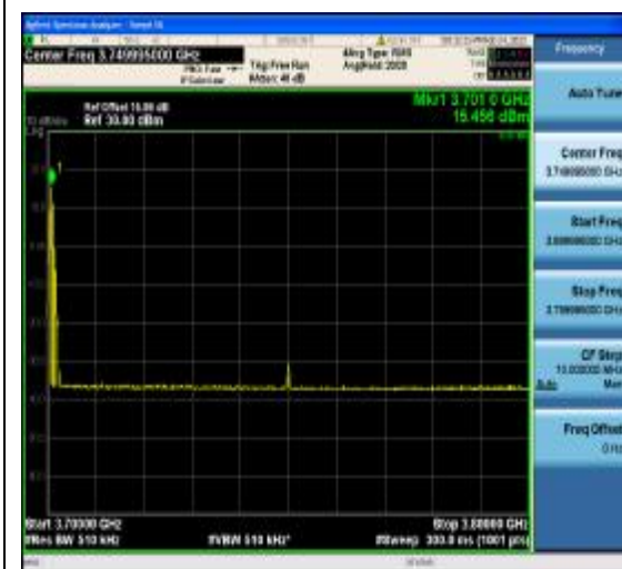
1-N77-3700-3980-PC2-30-100-L-4-CP-QPSK -Edge_1RB_Left-1@0-Ant1-3699.995~3799. 995(3700.995MHz,15.456MHz,Limit30,Margi n[14.544])-PASS-see graph
