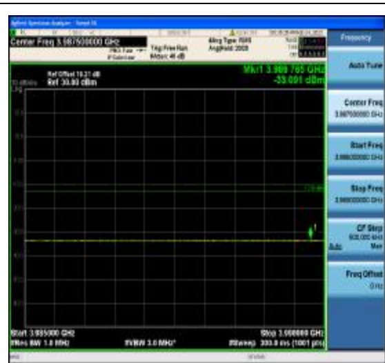
1-N77-3700-3980-PC2-30-100-H-3-DFT-PI2 BPSK-Outer_Full-270@0-Ant1-3985~3990(3 989.765MHz,-33.091MHz,Limit-13,Margin[20 .091])-PASS-see graph
