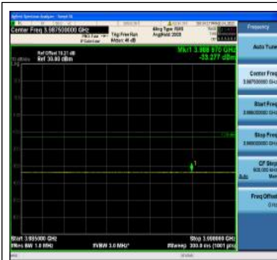
1-N77-3700-3980-PC2-30-100-H-2-DFT-PI2 BPSK-Edge_1RB_Right-1@272-Ant1-3985~ 3990(3988.97MHz,-33.277MHz,Limit-13,Mar gin[20.277])-PASS-see graph
