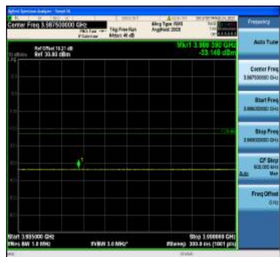
1-N77-3700-3980-PC2-30-100-H-6-CP-QPS K-Outer_Full-273@0-Ant1-3985~3990(3986. 39MHz,-33.148MHz,Limit-13,Margin[20.148]) -PASS-see graph
