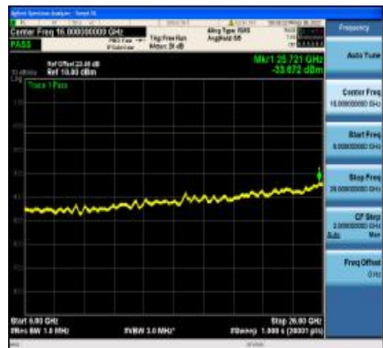
1-N77-3700-3980-PC2-30-20-L-7-DFT-16QA M-Edge_1RB_Left-1@0-6000-26000-Ant1--3 3.67--13-PASS
