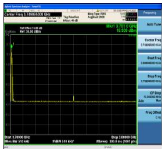
1-N77-3700-3980-PC2-30-100-L-6-CP-QPSK -Outer_Full-273@0-Ant1-3699.995~3799.995 (3700.995MHz,15.309MHz,Limit30,Margin[14 .691])-PASS-see graph
