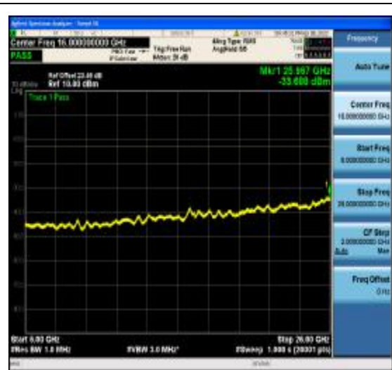
1-N77-3700-3980-PC2-30-20-H-3-DFT-PI2B PSK-Outer_Full-50@0-6000-26000-Ant1--33. 69--13-PASS
