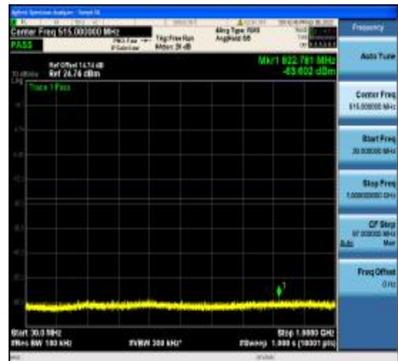
1-N77-3700-3980-PC2-30-20-H-2-DFT-PI2B PSK-Edge_1RB_Right-1@50-30-1000-Ant1-- 63.60--23-PASS
