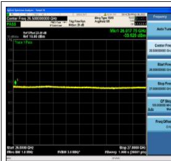
1-N77-3700-3980-PC2-30-20-H-1-DFT-PI2B PSK-Edge_1RB_Left-1@0-26000-40000-Ant 1--33.52--13-PASS
