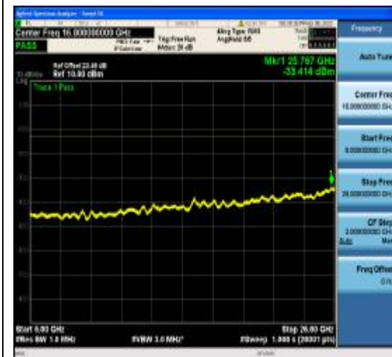
1-N77-3700-3980-PC2-30-20-L-16-CP-QPSK -Edge_1RB_Left-1@0-6000-26000-Ant1--33. 41--13-PASS
