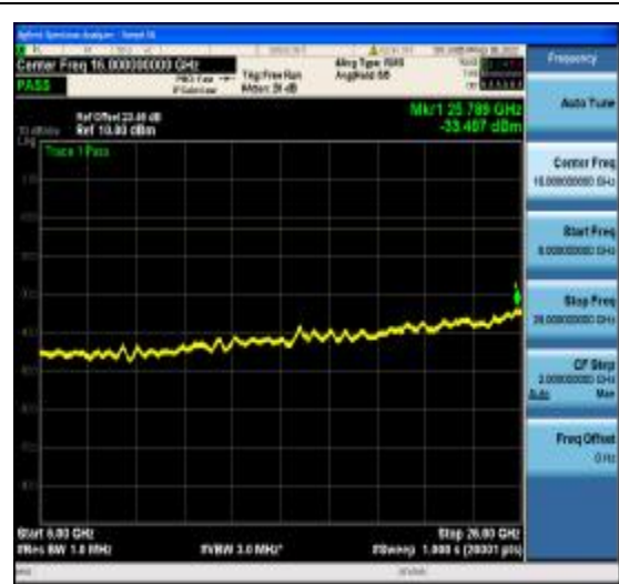
1-N77-3700-3980-PC2-30-20-M-14-DFT-256 QAM-Edge_1RB_Right-1@50-6000-26000-A nt1--33.49--13-PASS
