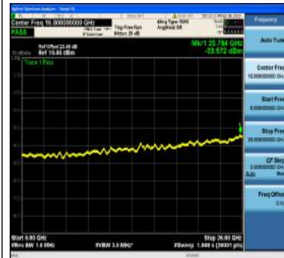
1-N77-3700-3980-PC2-30-20-M-13-DFT-256 QAM-Edge_1RB_Left-1@0-6000-26000-Ant1 --33.57--13-PASS
