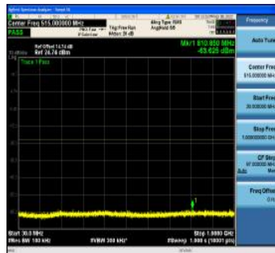
1-N77-3700-3980-PC2-30-20-M-14-DFT-256 QAM-Edge_1RB_Right-1@50-30-1000-Ant1- -63.63--23-PASS
