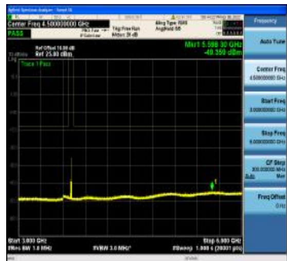
1-N77-3700-3980-PC2-30-20-L-26-CP-256Q AM-Edge_1RB_Right-1@50-3000-6000-Ant1 --49.36--13-PASS
