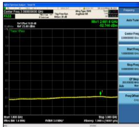
1-N77-3700-3980-PC2-30-20-M-14-DFT-256 QAM-Edge_1RB_Right-1@50-1000-3000-An t1--52.74--13-PASS
