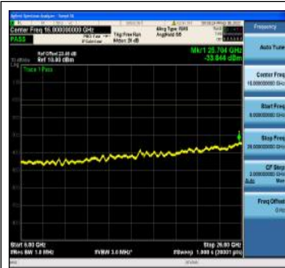
1-N77-3700-3980-PC2-30-20-M-11-DFT-64Q AM-Edge_1RB_Right-1@50-6000-26000-Ant 1--33.84--13-PASS
