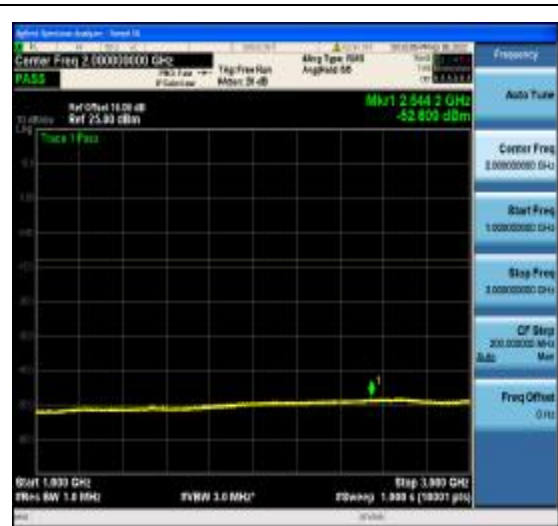
1-N77-3700-3980-PC2-30-20-M-8-DFT-16QA M-Edge_1RB_Right-1@50-1000-3000-Ant1-- 52.81--13-PASS
