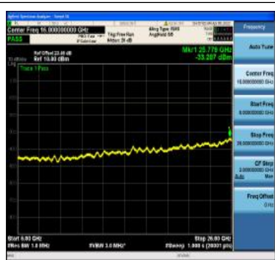
1-N77-3700-3980-PC2-30-80-M-7-DFT-16QA M-Edge_1RB_Left-1@0-6000-26000-Ant1--3 3.29--13-PASS
