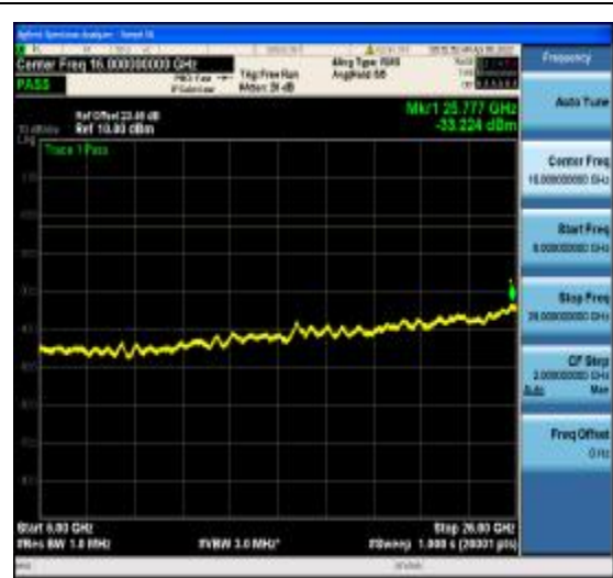
1-N77-3700-3980-PC2-30-80-H-8-DFT-16QA M-Edge_1RB_Right-1@216-6000-26000-Ant 1--33.22--13-PASS
